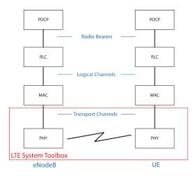
LTE Toolbox focuses on the physical layer, which is highlighted in red in the preceding figure. It also supports interfacing with portions of the RLC and MAC layers, which are highlighted in blue. The primary features of the LTE physical layer are OFDM modulation, including the time-frequency structure of the resource blocks, adaptive modulation and coding, hybrid-ARQ, and MIMO.
