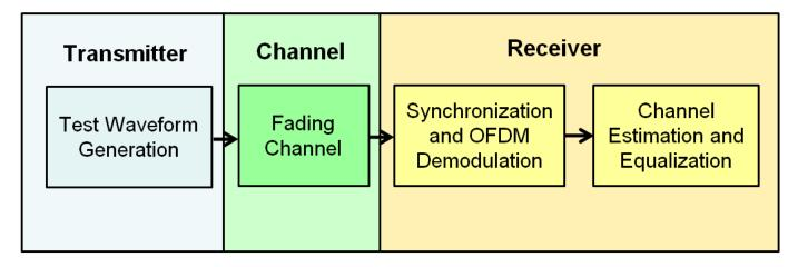
Generate an E-UTRA test model (E-TM) configuration. Use this configuration to generate the waveform and populate the resource grid.
