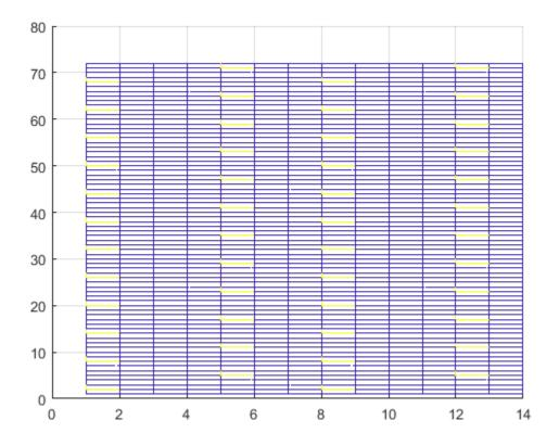
Alternatively, generate indices in subscript form by providing the 'sub' option string for lteCellRSIndices. In this case, the output indices represent the resource grid in the form [subcarrier, OFDM symbol, antenna port].
